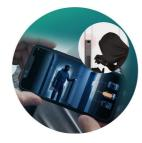
Philips Alpha-VP-5HWS equips with a wideangle camera and two low-power infrared fill lights. It has daytime mode and night vision mode. When the light is dim, the infrared fill light will automatically turn on, switch to night vision mode, and recognize the facial features within 1 meter from the lock end.
