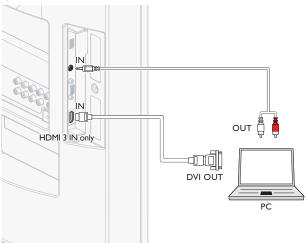
If you connect a PC with an HDMI or Display Port (HDMI-Display Port conversion cable) connector.
