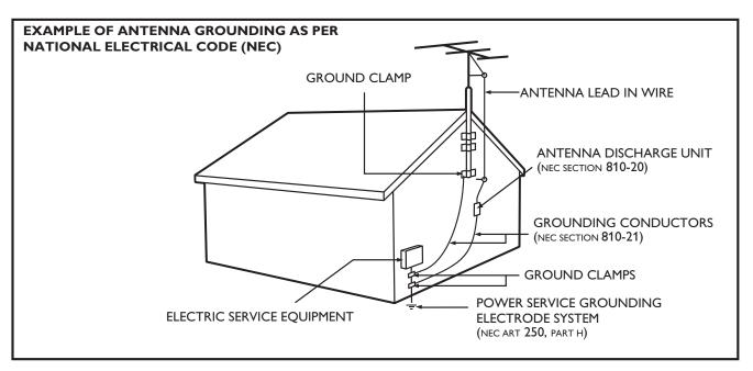
**Note to the CATV system installer:** this reminder is provided to call the CATV system installer's attention to Article 820-40 of the NEC that provides guidelines for proper grounding and, in particular, specifies that the cable ground shall be connected to the grounding system of the building, as close to the point of cable entry as practical.
