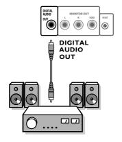
Connect a Digital MultiChannel Surround receiver to the **DIGITAL AUDIO OUT** connector at the bottom of the TV.
