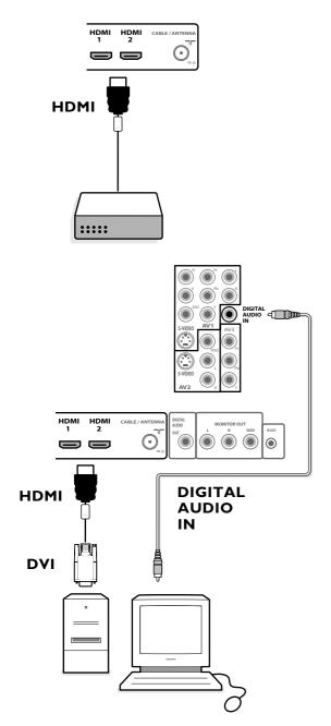
HDMI is the leading new standard for Digital video and audio interconnection. To the **HDMI** connector you can connect HDMI devices such as a Set Top Box or compatible DVD-R or DVD player with HDMI, or DVI-equipped devices like a computer.
