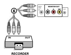
The **MONITOR OUT** connector can be used for a daisy chaining or to record programs from your TV **(()**. Only when a recorder is connected to **MONITOR OUT** it is possible to record an analog program from your TV. See Record with your recorder, p. 37.
