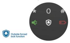
Before leaving home, you can touch the outside forced lock button to enable the function. In this mode, opening the door from inside will trigger an alert. This feature can effectively remind you of security risks and upgrade the level of home security.
