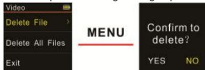
If the device shows the interface on the left side, select “+” or “-” button to choose to delete single file or all files. If the device shows the interface on the left side, select “YES” to confirm deleting or “NO” to retain file by “◀◀” or “▶▶” button. Press Menu button to execute the option.
