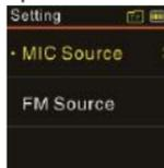
If the "FM Source" is selected, the radio will be the sour for voice recording. Press Menu button to set the frequency point.
