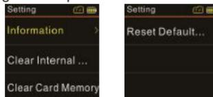
Information: users can check the device's firmware version and check the remaining capacity of memory by using this function.
