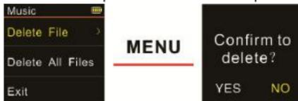
If the device shows the interface on the left side, press "+" or "-" button to select individual or all files; if the device shows the interface on the right side, press "⏪" and "⏩" to choose "YES" to confirm deletion, "NO" to keep file; press MENU button to execute.
