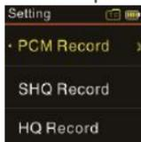
HPCM REC: WAV format, high sound quality, bit rate: 3072kbps.
