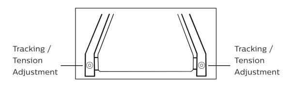
Note: Adjustment is through small hole in the end cap.
