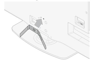
2 Pass cables through the cable management tie to avoid tangles.
