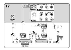
If your recorder has an S-VHS video jack: for improved picture quality, connect a S-Video cable with the **S-VIDEO** input and connect the audio cables to the **AUDIO L** and **R** input jacks of **AV1**.
