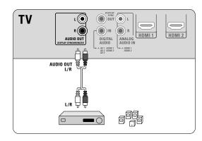
Due to legal requirements, it is possible that with certain copy protected PCM audio qualities from a accessory device connected to the **HDMI** input, the Digital audio signal is muted.
