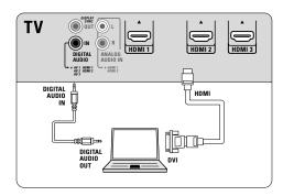
11.3.4 Equipped with a HDMI connector
