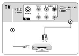
When using the S-VIDEO connector, do not connect any device to the AV VIDEO input that you are using.
