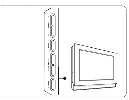
Press the **POWER** () switch to turn the TV on. The **MENU** button can be used to summon or exit the TV menu without the remote control.
