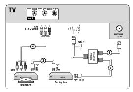
11.9 Connect a satellite receiver or Set top box with A/V outputs
