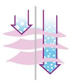
The ionisation process creates smaller steam particles that reach deeper into the fabric. This means even the toughest creases are removed easily.
