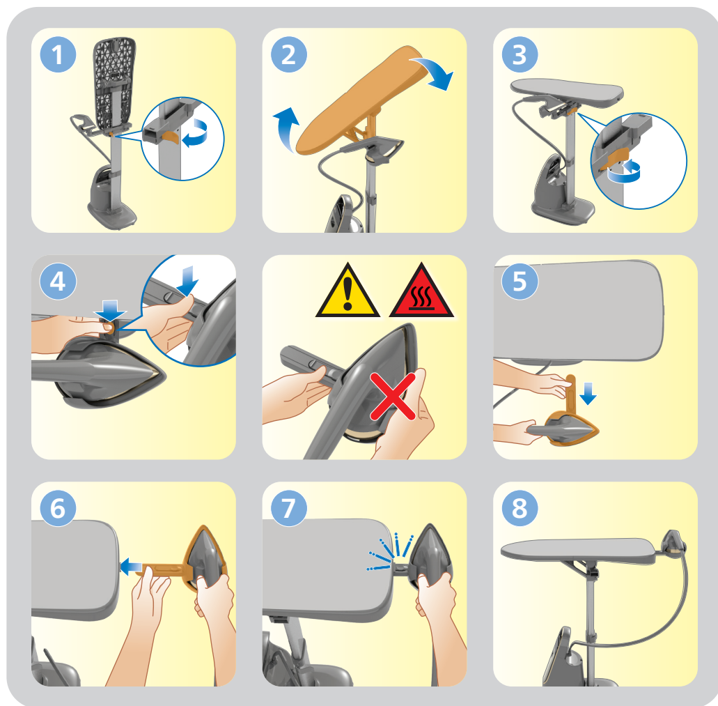
EN Figure 1: Unlock the 2nd clip from the top. Figure 2: Push the board down to horizontal position. Figure 3: Lock the clip.
