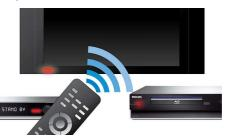
EasyLink uses the HDMI CEC industry standard protocol to share functionality between connected devices and the TV. With EasyLink only one remote control is needed to operate the main functionalities on your TV and connected devices. EasyLink uses a standard HDMI cable to transfer system commands. It works between all electronic devices equipped with HDMI CEC.
