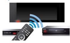
EasyLink uses the HDMI CEC industry standard protocol to share functionality between connected devices and the TV. With EasyLink only one remote control is needed to operate main functionalities on your TV and connected devices. EasyLink uses the standard HDMI cable to transfer system commands. It works between all electronic devices equipped with HDMI CEC.
