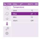
**3** You can select the alert option to turn on the alert. To change the maximum and minimum temperatures for the temperature alert, select the desired temperatures at 'Max' and 'Min' in the temperature menu.
