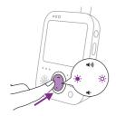
1 Press the left or right part of the control button to adjust the brightness. This will adjust both the brightness of the display and lights of the parent unit at the same time.
