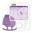
When sound is picked up by the baby unit, the display and sound of the parent unit switch on immediately. The sounds are transmitted to the parent unit and the sound level lights light up green. As long as no sound is detected, the sound level lights are off.
