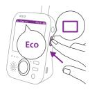
Press the mode button on the side of the parent unit to switch to Eco mode.
