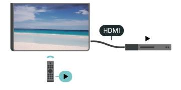
HDMI CEC (Consumer Electronic Control) must be switched on on the TV and the connected device.
