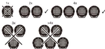
If an additional pair of position lights is not permitted, the position light should be disconnected. The legal regulations in individual countries must be observed.
