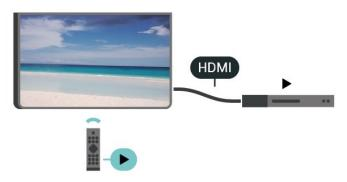
HDMI CEC (Consumer Electronic Control) must be turned on on the TV and the connected device.
