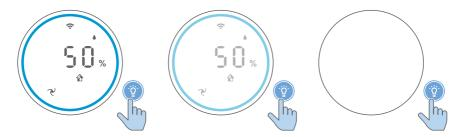
With the light sensor, the control panel can automatically turn on, turn off or dim according to the ambient light. The control panel will be off or dim when the ambient light is dark. You can touch any button to wake up all lights and check the air quality. Then, if no further operation, all lights will be off or dim again to match with the ambient light.
