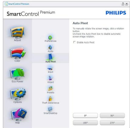
**Options>Input** - Will only be active when selecting Input from the drop-down Options menu. On a non-supported display capable of DDC/CI, only the Help and Options tabs are available. All other SmartControl Premium tabs are not available.
