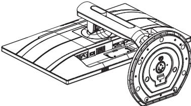
3. While keeping the release button pressed, tilt the base and slide it out.
