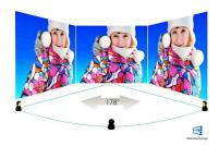
AH-IPS displays use an advanced technology which gives you extra wide viewing angles of 178/178 degree, making it possible to view the display from almost any angle. Unlike standard TN panels, AH-IPS displays gives you remarkably crisp images with vivid colors, making it ideal not only for Photos, movies and web browsing, but also for professional
