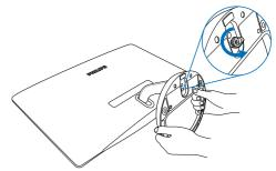
2. Release the screw of base stand then pull the base away from the monitor.
