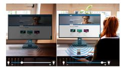
PowerSensor is a built-in 'people sensor' that transmits and receives harmless infrared signals to determine if user is present and automatically reduces monitor brightness when user steps away from the desk, cutting energy costs by up to 70 percent and prolonging monitor life.
