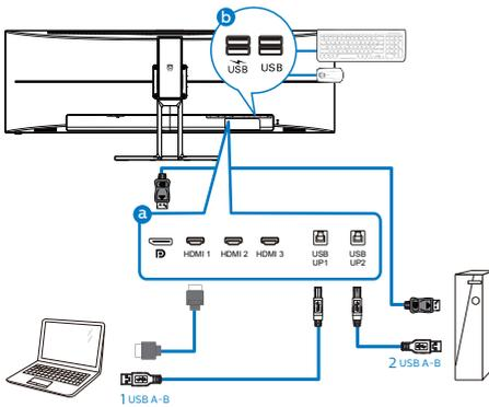
3. Enter to OSD menu. Go to KVM layer and select “USB up1” or “USB up2” to switch the control of peripherals from one device to another. Simply repeat this step for switching the control system using one set of peripheral.
