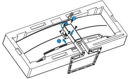
3. After attaching the base, erect the monitor with both hands on holding the monitor together with styrofoam firmly. Now you can pull out the styrofoam. Notice this monitor is curved design, when you pull out styrofoam, do not squeeze the panel to avoid broken panel.
