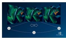
IPS displays use an advanced technology which gives you extra wide viewing angles of 178/178 degree, making it possible to view the display from almost any angle. Unlike standard TN panels, IPS displays gives you remarkably crisp images with vivid colors, making it ideal not only for Photos, movies and web browsing, but
