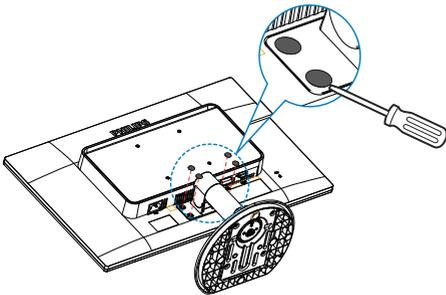
3. Remove the screws from hinge cover.
