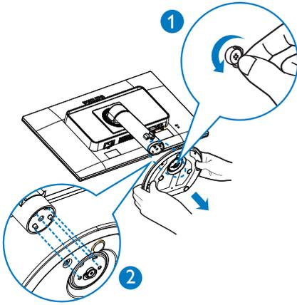
3. While keeping the release button pressed, tilt the base and slide it out.
