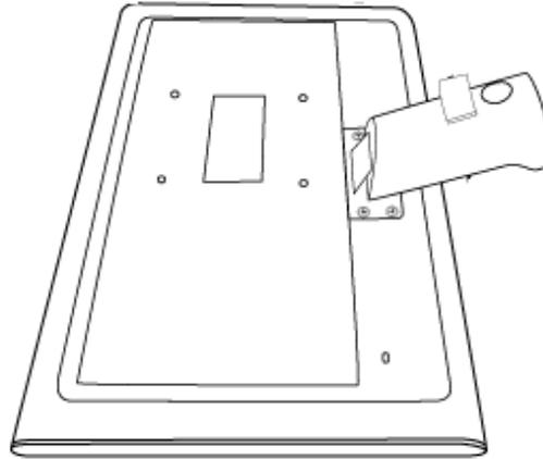
2) Hold the monitor base with both hands and firmly insert the base stand into the base column.
