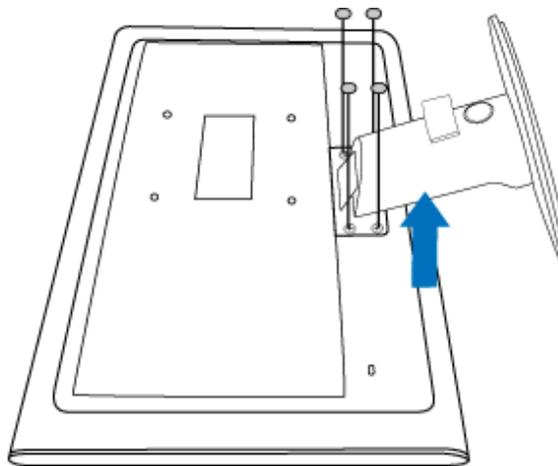
Remove the 4 screws and then remove the base from the LCD monitor.
