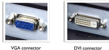
Dual input provides connectors to accommodate input of both analog VGA and digital DVI signals.
