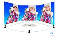
Philips MVA LED display uses an advanced multi-domain vertical alignment technology which gives you super-high static contrast ratios for extra vivid and bright images. While standard office applications are handled with ease, it is especially suitable for photos, webbrowsing, movies, gaming, and demanding graphical applications. It's optimized pixel management technology gives you 178/178 degree extra wide viewing angle, resulting in crisp images.
