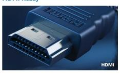
An HDMI-ready device has all the required hardware to accept High-Definition Multimedia Interface (HDMI) input. A HDMI cable enables high-quality digital video and audio all transmitted over a single cable from a PC or any number of AV sources (including set-top boxes, DVD players, A/V receivers and video cameras).
