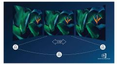
IPS displays use an advanced technology which gives you extra wide viewing angles of 170/170 degree, making it possible to view the display from almost any angle. Unlike standard TN panels, IPS displays gives you remarkably crisp images with vivid colors, making it ideal not only for Photos, movies and web browsing, but also for professional applications which demand color accuracy and consistent brightness at all times.
