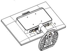
2. Use a flathead screwdriver to remove four mylars from the hinge cover.
