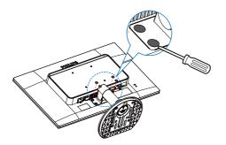
3. Remove the screws from hinge cover.
