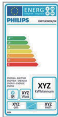
The European Energy Label informs you on the energy efficiency class of this product. The greener the energy efficiency class of this product is the lower the energy it consumes. On the label, you can find the energy efficiency class, the average power consumption of this product in use and the average energy consumption for 1 year.
