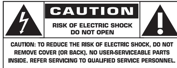
**CAUTION:** TO REDUCE THE RISK OF ELECTRIC SHOCK, DO NOT REMOVE COVER (OR BACK). NO USER SERVICEABLE PARTS INSIDE. REFER SERVICING TO QUALIFIED SERVICE PERSONNEL.
