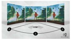
Philips VA LED display uses an advanced multidomain vertical alignment technology which gives you super-high static contrast ratios for extra vivid and bright images. While standard office applications are handled with ease, it is especially suitable for photos, web-browsing, movies, gaming, and demanding graphical applications. It's optimized pixel management technology gives you 178/178 degree extra wide viewing angle, resulting in crisp images.
