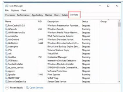
3. Scroll down and select ‘WbioSvc’ (Windows Biometric Service). If the status shows ‘Running’, right click to stop the service first, then restart the service manually.
