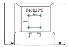
2. Remove the 4 screws and then remove the base from the monitor.
