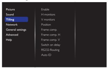
Create a single large-screen matrix (video wall) that consists of up to 100 sets of display (up to 10 sets in vertical side and 10 sets on the horizontal side).
