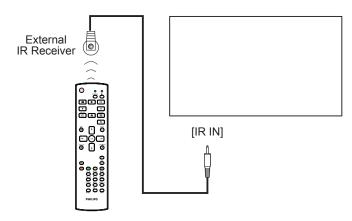
NOTE: The remote control sensor of this display will stop working if the [IR IN] is connected.
