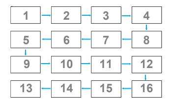
**Note 1**: To use this function, serially connect all machines with RS-232 cable and set their Network control port to RS-232.
