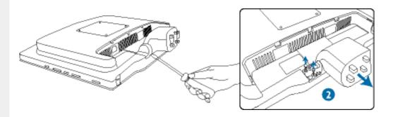
2) Remove the screws and then detach the base attachment unit from the LCD monitor.
