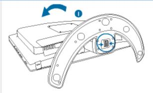
1) Place the monitor face down a smooth surface taking care to avoid scratching or damaging the screen.
