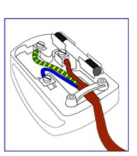
Before replacing the plug cover, make certain that the cord grip is clamped over the sheath of the lead - not simply over the three wires.
