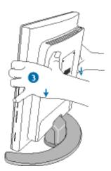
3) Firmly fix screen into the base plate.
