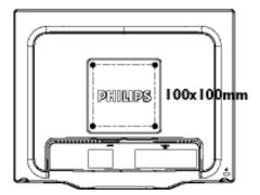
Note: This monitor is designed to work with a 100mm x 100mm VESA-compliant mounting interface.
