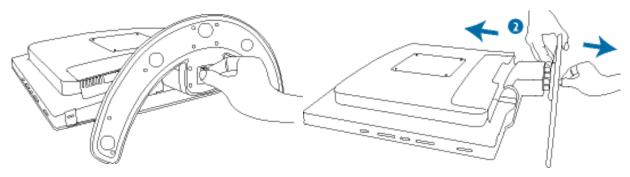
2) Press the release latches on the bottom of the base together and gently remove the attachment unit from the base.
