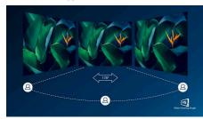
IPS displays use advanced technology that gives you extra-wide viewing angles of 178/178 degrees, making it possible to view the display from almost any angle - even in 90-degree Pivot mode! Unlike standard TN panels, IPS displays gives you remarkably crisp images with vivid colours, making it ideal not only for Photos,
