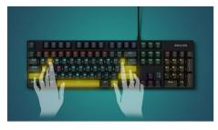
Fast complex gaming key strokes demand advanced performance. With full N-key rollover every key is registered independently without confusion so that each keystroke is correctly registered regardless of how many other keys are being pressed or held down at the time.
