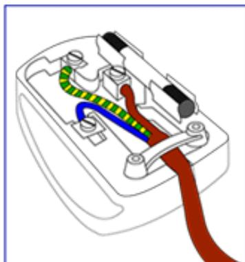
1. The GREEN AND YELLOW wire must be connected to the terminal in the plug which is marked with the letter "E" or by the Earth symbol  $\perp$  or coloured GREEN or GREEN AND YELLOW.
