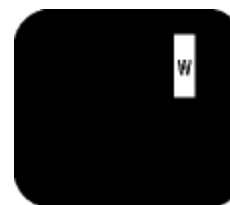
Three adjacent lit sub pixels (one white pixel)
