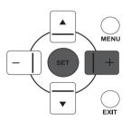
3. Press the **PLUS/SET** button to enter the submenu.
