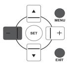
5. Press the **MINUS/EXIT** button on the remote control to return to the previous menu, or press the **MENU** button to exit the OSD menu.
