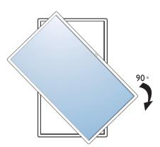
Note: The remote control sensor should be on the right side when rotating your display.
