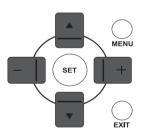
4. In the submenu, press the **UP/DOWN** button to toggle between items, or press **PLUS/MINUS** button to adjust settings. If there is a submenu, press the **PLUS** button to enter it.
