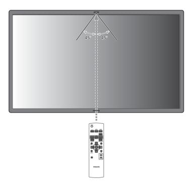
Note: The remote control may not function properly if the remote control sensor on the display is under direct sunlight, in a location with strong illumination, or if there is an obstacle in the path of signal transmission.
