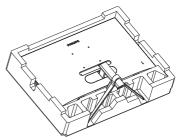
2. Remove the hinge cover from monitor body by using auxiliary tool.
