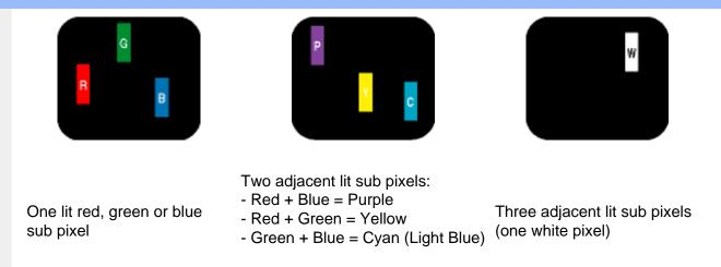
Black Dot Defects appear as pixels or sub pixels that are always dark or 'off'. These are the types of black dot defects:
