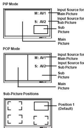
In PIP mode, a small window is displayed in one of the four corners. The OSD on the upper right corner will denote the input selected for main picture (large screen) and the sub-picture (small screen) displayed.
