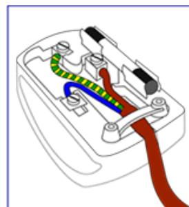
1. The GREEN AND YELLOW wire must be connected to the terminal in the plug which is marked with the letter "G" or by the Ground symbol  $\pm$  or coloured GREEN or GREEN AND YELLOW.
