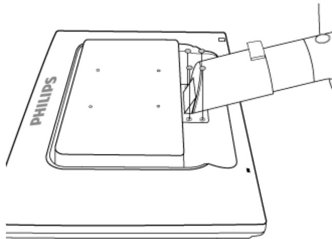
**(b)** Remove the 4 screws and then remove the base from the LCD monitor.
