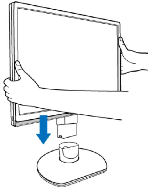
**(c)** Attach the monitor stand to the monitor column until the tabs "click" into place before releasing the height adjustable column.
