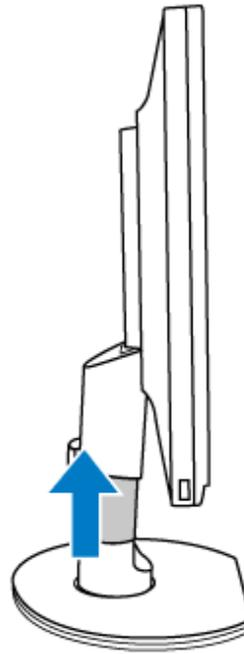
**(b)** Place the monitor face down on a smooth surface, taking care to avoid scratching or damaging the screen. Then lift the monitor stand.
