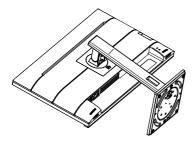
While keeping the release button pressed, tilt the base and slide it out.
