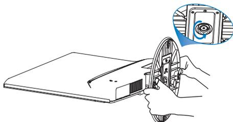
2. Release the screw of base stand then pull the base away from the monitor:
